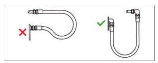
Where the radius falls below the required minimum, an angle adapter should be used as shown above to avoid sharp bends in hose.
