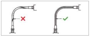
Hose should not be twisted. Hose is weakened when installed in twisted position. Also pressure in twisted hose tends to loosen fitting connections. Design so that machine motion produces bending rather than twisting.
