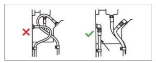
Obtain direct routing of hose through use of  $45^\circ$  and  $90^\circ$  adapters and fittings. Improve appearance by avoiding excessive hose length.
