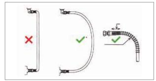
\* Never use a banding radius less than the minumum amount shown in the table. To prevent twisting and distortion, hose should be bent in the same plane as the motion of the boss to which the hose is connected.
