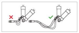
Adequate hose length is most important to distribute movement on flexing applications and to avoid abrasion.
