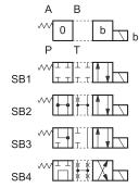
Type **TB**: 1 solenoid side B 2 external positions with return spring
