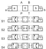
Type **RK**: 2 solenoids - 2 positions with mechanical retention
